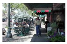
Typical sidewalks in mixed-use commercial areas should be 12-16 feet wide to encourage outdoor seating while providing adequate passing clearance.
